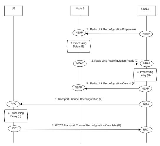
Figure 1. Signalling for Gating Initiation or Termination when SRNC=CRNC
