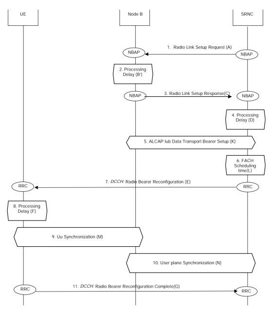
Figure 2. Signalling for transition from CELL\_FACH to CELL\_DCH
