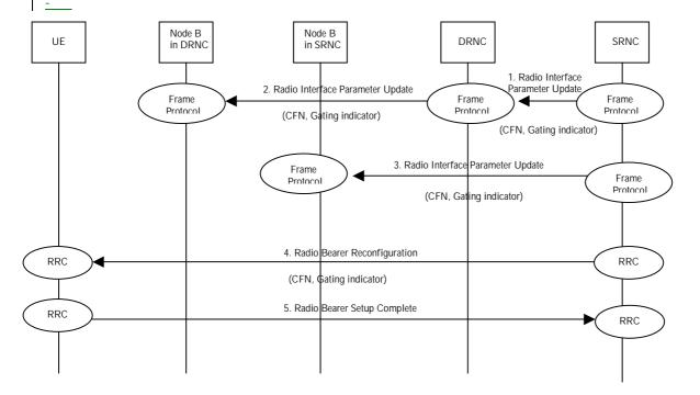
1. SRNC initiates/terminates gating operation sending Radio Interface Parameter Update Control Frame to DRNC with CFN and gating indicator.
