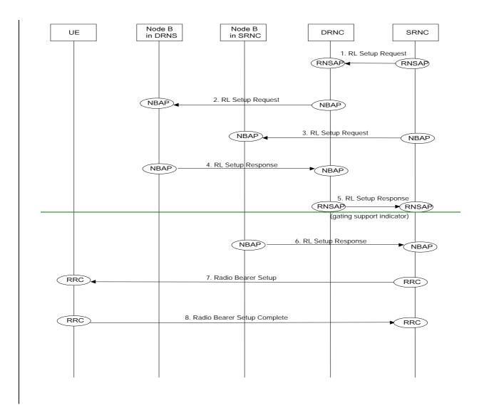
1. When SRNC sets up a Radio Link via the DRNC, SRNC sends **Radio Link Setup Request** message to DRNC with gating parameters.
