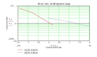
Figure 1: Comparison of CLPC-FACH and OLPC-FACH versus FER (Perfect OLPC): 40 ms TTI/ 5Hz
