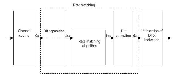
Figure 8: Rate matching for uncoded TrCHs, convolutionally encoded TrCHs, and for turbo encoded TrCHs with repetition in downlink
