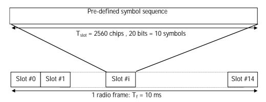
Figure 13: Frame structure for Common Pilot Channel
