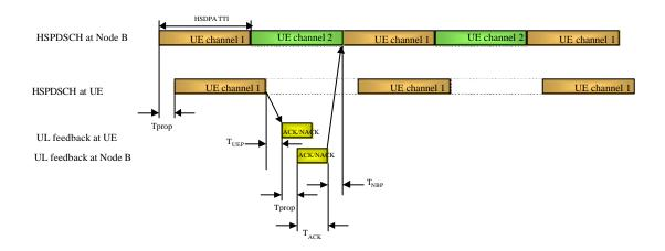
Figure 28. Timing relations for 2-channel HARQ process
