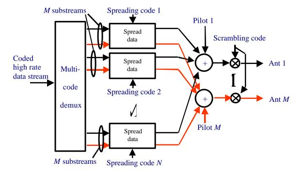
Figure 6. Block diagram of MIMO transmitter
