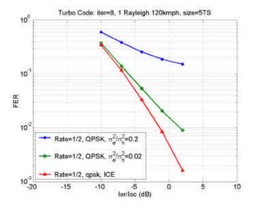
Figure 57 FER versus Ior/Ioc , R=1/2 QPSK, 120 kmph
