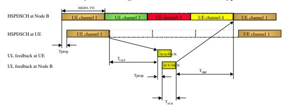
Figure 29. Timing relations for 4-channel HARQ process
