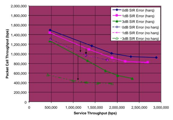
**Figure 26.** Packet Throughput vs Service Throughput w/wo H-ARQ for different CPICH SIR Measurement Errors using a Max C/I Scheduler.
