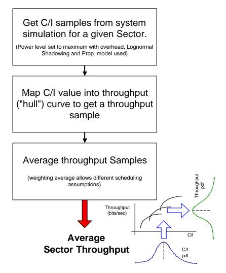
Figure 76. Analytic Simulation Flow Chart
