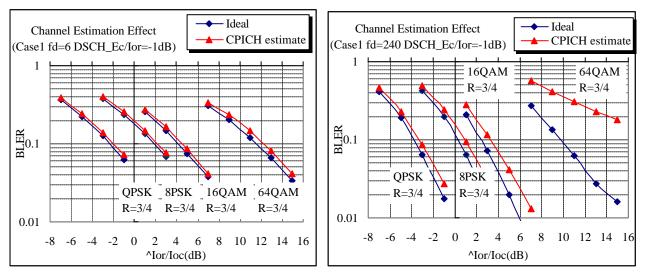
Figure 15 Performance degradation due to Phase/Amplitude estimation error
