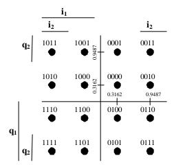
Figure 44. Signal Constellation for 16-QAM Modulation.
