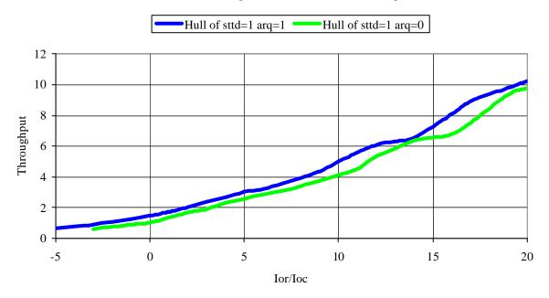
Figure 52. Hull curves at 3 kmph with and without HARQ
