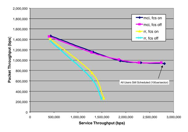
Figure 34. Packet Throughput vs Service Throughput for Max C/I and Round Robin
