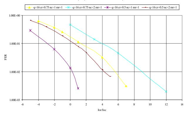
Figure 48. FER vs. Ior/Ioc for 16 QAM- Flat Fading @ 3Kmph
