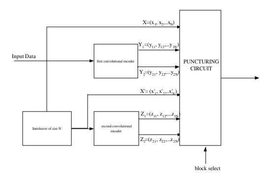
Figure 18. Block Diagram of a Turbo Encoder
