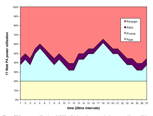
**Figure 72** Percentage utilization of 17 Watt PA for a given sector in the system. Note at all times 17 Watts is transmitted for each sector.
