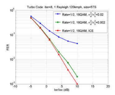
Figure 59 FER versus Ior/Ioc , R=1/2 QAM, 120 kmph.
