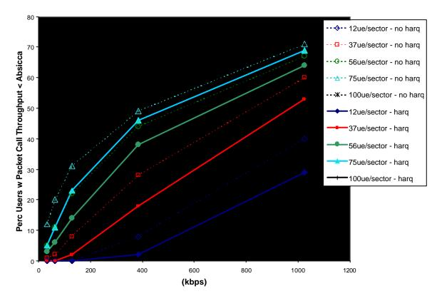
**Figure 24.** %User Packet Call Throughput CDF w/wo H-ARQ for the 1dB CPICH SIR measurement error case using a Max C/I Scheduler
