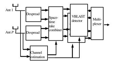
Figure 7. Block diagram of a MIMO receiver
