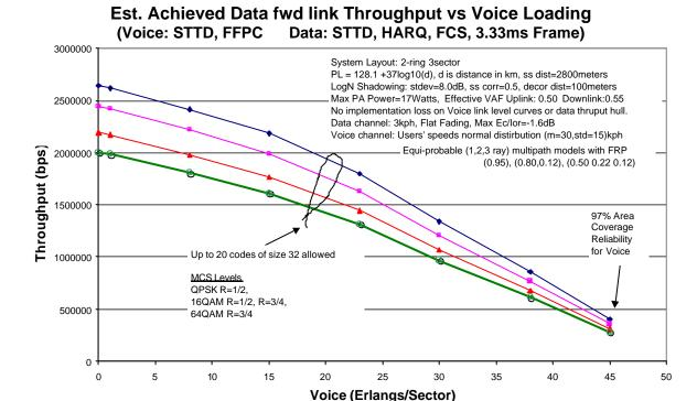
Figure 69 HSDPA Throughput vs Voice Loading for different FRP (lamda) where an Equal Average Power Scheduler is assumed
