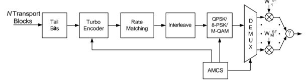
Figure 4. HSDPA Physical Layer Structure
