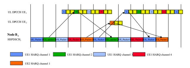
Figure 5. Principle of N-channel stop-and-wait HARQ (N=4).
