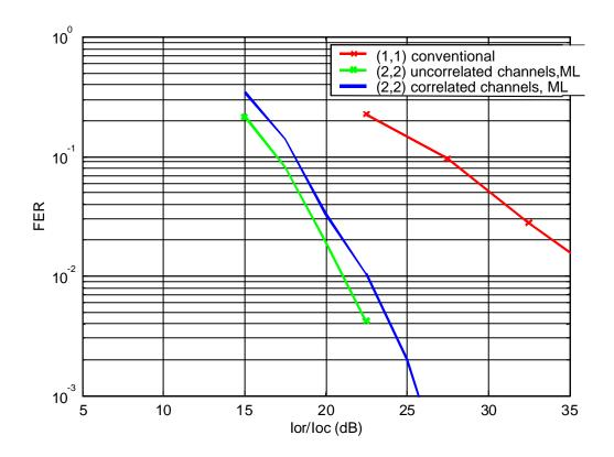
Figure 38. FER for (2,2) system, 10.8 Mbps, flat channel, 3km/hr
