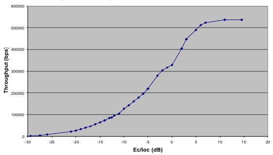
Figure 68. HSDPA Throughput Hull Curve vs Ec/Ioc for 3kph and flat fading
