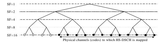
$SF_{HSDPA} = 16$  (example) Number of codes to which HSDPA transmission is mapped: 12 (example)
