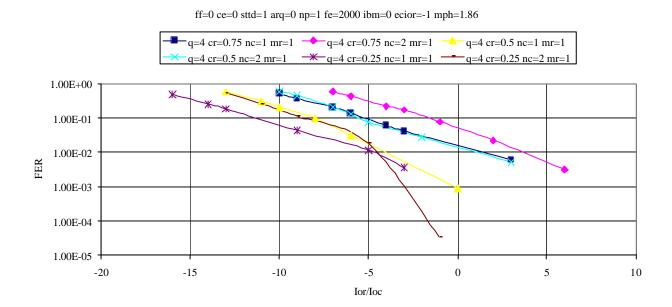
Figure 47. FER vs. Ior/Ioc for QPSK - Flat Fading @3 kmph
