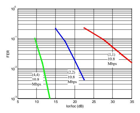
Figure 36. Flat fading channel performance for 10.8 Mbps
