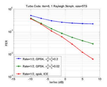
Figure 56. FER versus Ior/Ioc, R=1/2 QPSK, 3 kmph
