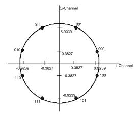
Figure 43. Signal Constellation for 8-PSK Modulation.
