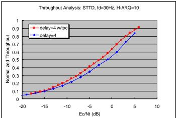
**Figure 75** Delay compensation with TPC (ARQ=10: TPC error rate=3%)
