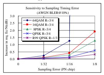
Figure 14. Performance degradation due to sample timing error
