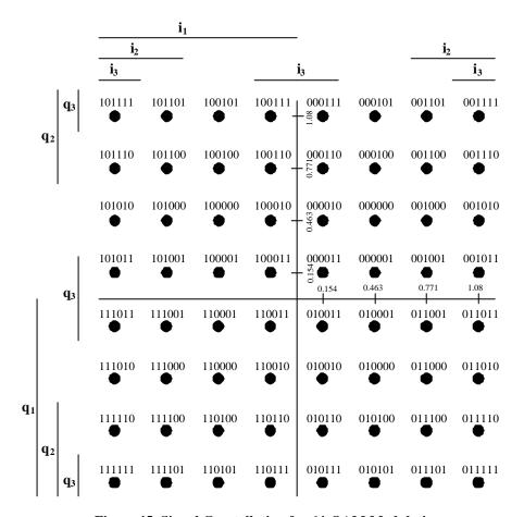
Figure 45. Signal Constellation for 64-QAM Modulation.
