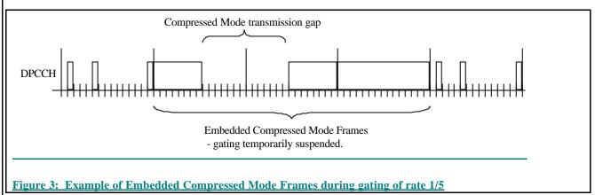
The UTRAN may therefore use the uplink TFCI to detect the presence of Embedded Data Periods during Embedded Compressed Mode Frames.
