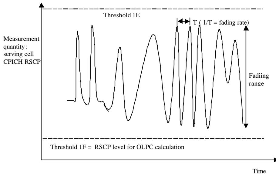
Figure 1: Primary CPICH RSCP fading range measurement
