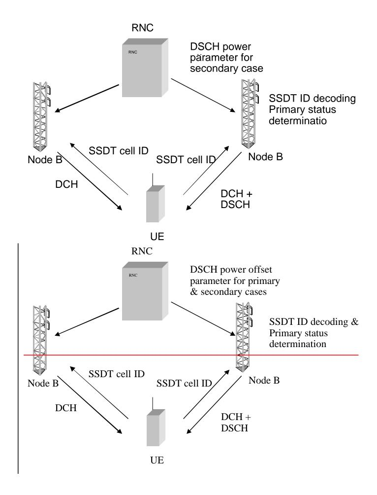
Figure 1. Concept of using SSDT signalling with DSCH power control
