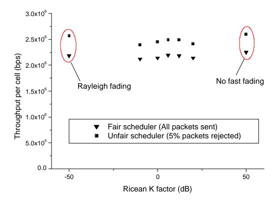
Figure 1 Effect of fast fading model on throughput
