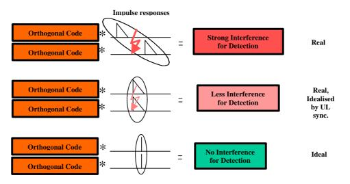
Figure 1 The performance improvement mechanism of UL synchronization control
