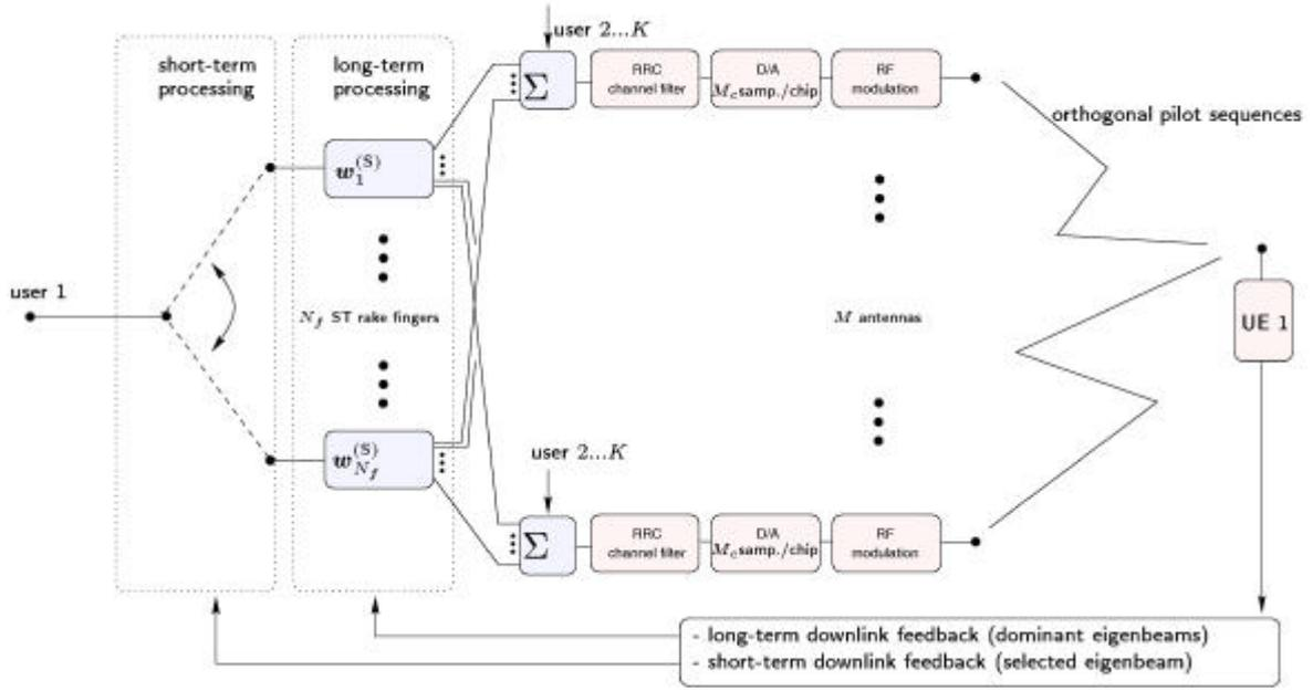
Figure 3: Structure of the downlink eigenbeamformer
