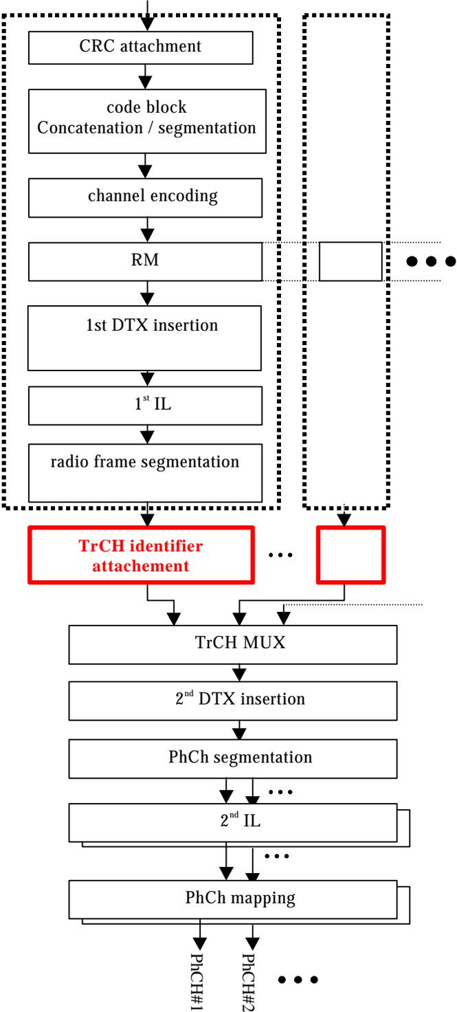
So each symbol  $s$  in  $\{0,1,\delta\}$  is replaced by a 2-tuple  $(s,i)$  where  $s$  is the symbol and  $i$  the TrCH id.  $i$  is from 1 to  $I$  for TrCH bits  $\{0,1\}$  and  $i$  takes the special value 0 for DTX indicators.
