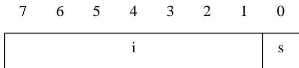
When this is a DTX symbol, the octet is zero, that is to say all the bits are zero. When this is a bit  $s$  in  $\{0,1\}$ , the parity bit tells the value of  $s$ , whereas the bits from weigh 1 up to 7 tells the value of  $i$  in  $\{1, 2, \dots, I\}$
