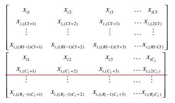
(4) Perform the inter-column permutation based on the pattern { $P_1(j)$ } (j=0,1, ...,  $C\underline{I}$ -1) shown in table 3, where  $P_1(j)$  is the original column position of the j-th permuted column. After permutation of the columns, the bits are denoted by  $y_{ik}$ ; from the first column of the first row and ending with bit in column  $C_I$  of row  $R_J$ , and excluding any positions that is marked as a "p-bit". For instance when no position is marked as a p-bit we get the following :
