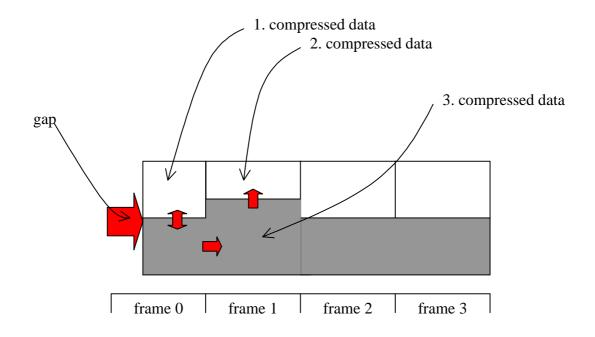
Figure 1 Example of compressed mode with several TTI durations
