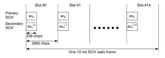
Figure 16: Structure of Synchronisation Channel (SCH)
