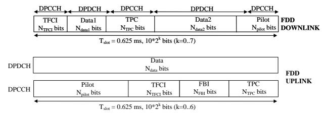
Figure 7. The slot content for the DPDCH/DPCCH. The exact bit allocations are not shown.
