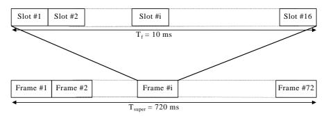
Figure 6. Basic frame structure.
