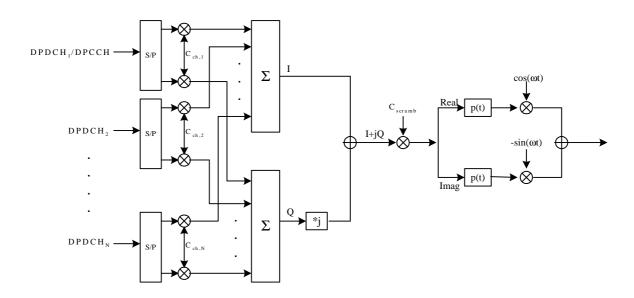
Figure 9. Spreading/modulation for downlink DPCH.
