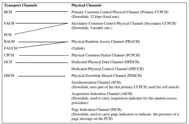
Figure 5: Transport-channel to physical-channel mapping.
