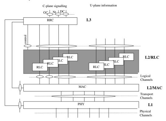
Figure 2. Radio interface protocol architecture of the RRC sublayer, L2 and Physical layer (L1).
