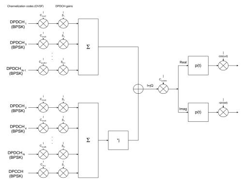
Figure 8. Spreading/modulation for uplink DPDCH/DPCCH for user services less than or equal to 1024kbps in the 5MHz band
