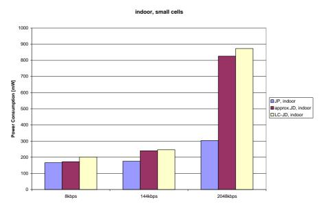
Fig.3: overall power consumptions in the indoor environment in small cells.
