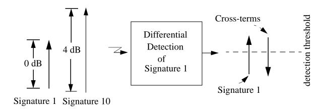
Figure 1: Result of differential detection when two signatures are present.
