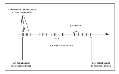
Figure 5. Typical characteristic of a packet service session
