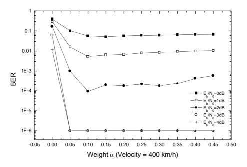
Fig 5. Receiver Performance at Velocity of 400 km/h
