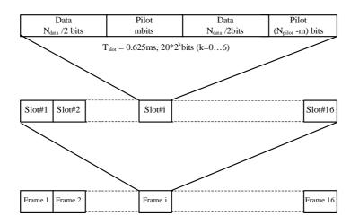
Fig. 2 Proposed Slot and Frame Structure
