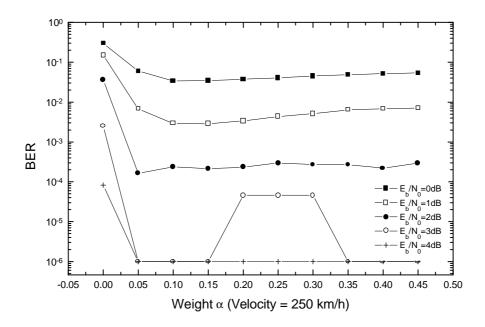
Fig.4 Receiver Performance at Velocity of 250 km/h
