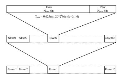
Fig.1 Current Frame Structure
