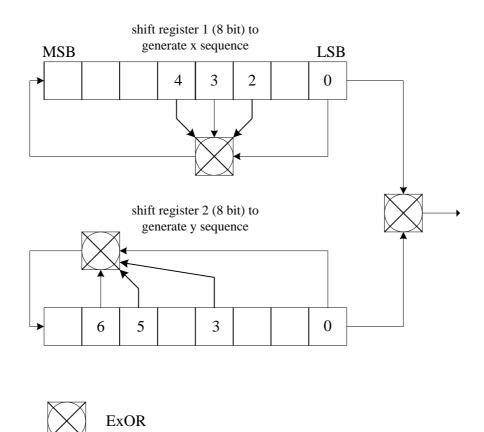
Figure 8. Preamble spreadingcode generator
