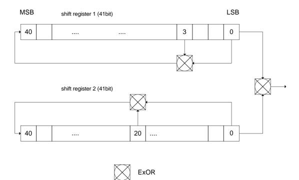
Figure 5. Configuration of uplink scrambling code generator
