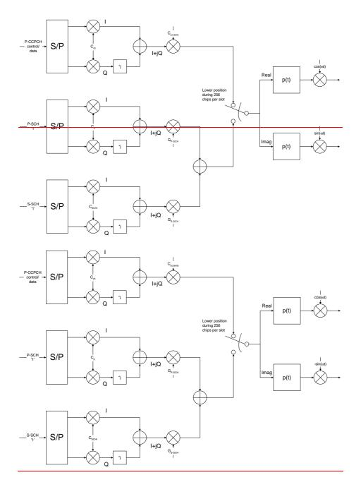
Figure 11. Spreading and modulation for SCH and P-CCPCH
