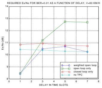
Figure 2: Required Es/N0 for BER=0.01 as a Function of Uplink/Downlink Delay. V=60 km/h.
