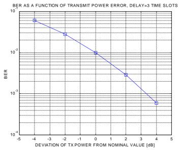
Figure 3: BER as a function of Transmit Power Deviation from Nominal Value. Delay=3 Time-Slots.
