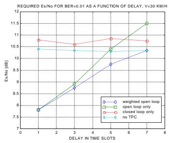
Figure1: Required Es/N0 for BER=0.01 as a Function of Uplink/Downlink Delay. V=30 km/h.
