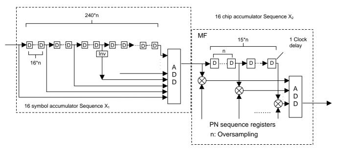
Figure 3: Efficient Correlator for plain hierarchical sequence.
