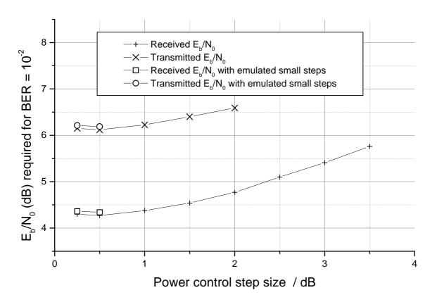
Figure 2 Eb/No for BER=0.01, terminal speed 1km/hr, 6 path channel
