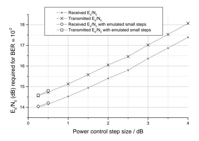
Figure 1: Eb/No for BER=0.01, terminal speed 300km/hr, single path
