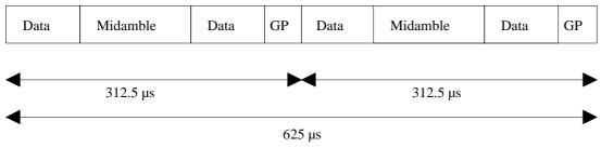
Figure 5: Double RACH burst structure
