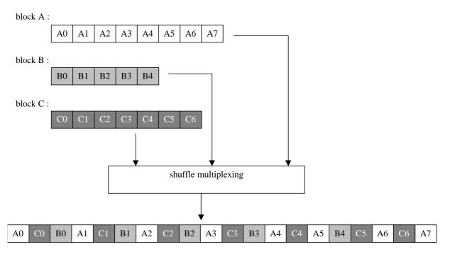
Figure 5 Shuffle Multiplexing
