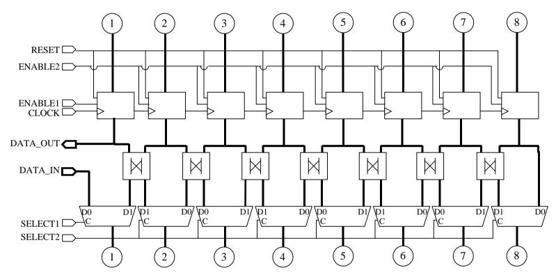
Figure 4 Hardware accelerator for fonction « find j such that  $e_j = min \{e_1, e_2, \dots, e_8\}$  »
