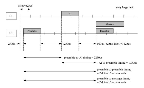
Fig.4 Timing of AICH transmission/reception (very large cell)
