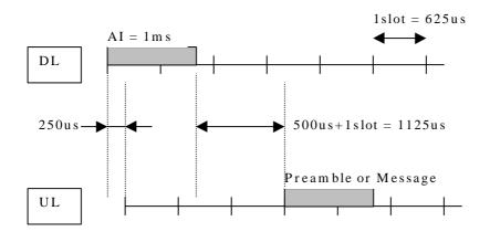
Fig.2 Minimum timing from AI to Preamble/Message
