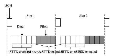
Figure: STTD encoding for the data symbols of the PCCPCH is shown.
