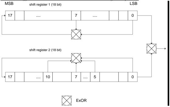
Figure 12. Configuration of downlink scrambling code generator
