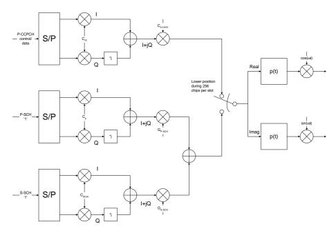
Figure 11. [Multiplexing of SCH]{Transmission of PCCPCH}
