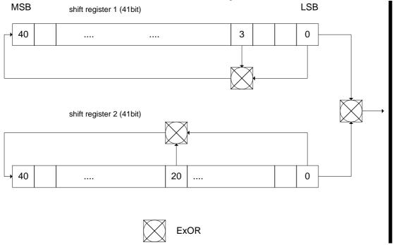
Figure 5. Configuration of uplink scrambling code generator
