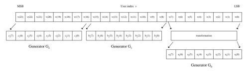
Figure 7. Uplink short scrambling code generator state initialisation
