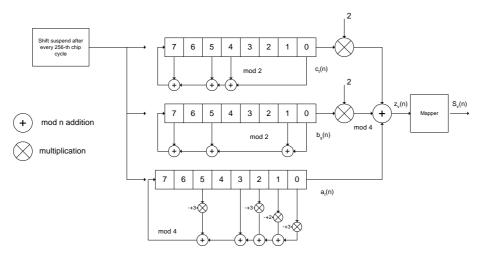
Figure 6. Uplink short scrambling code generator
