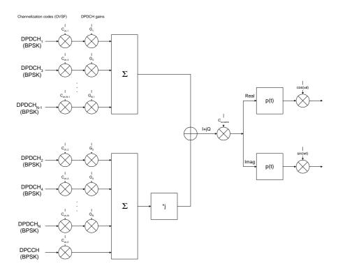
$Figure \ 1 \quad Spreading/modulation \ for \ uplink \ DPDCH/DPCCH \ for \ user \ services \ less \ than \ or \ equal \ to \ 1024kbps \ in \ the \ 5MHz \ band$
