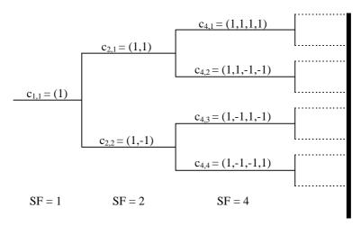
Figure 3. Code-tree for generation of Orthogonal Variable Spreading Factor (OVSF) codes.
