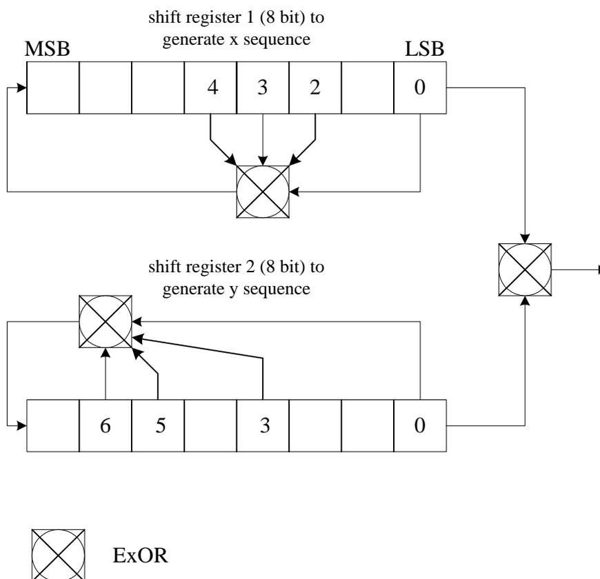
**Figure 8. Preamble ~~spreading~~~~scrambling~~ code generator**
