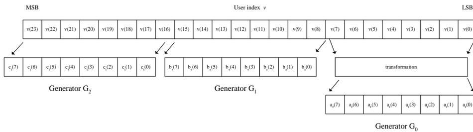
Figure 7. Uplink short scrambling code generator state initialization
