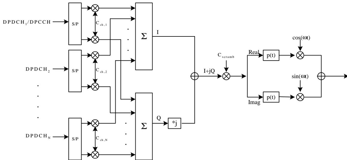
**Figure 10. Spreading/modulation for downlink DPCH and CCPCHs.**
