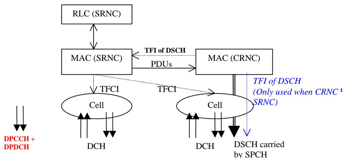
Figure 1. DSCH & DCH operation from network side with different SRNC & CRNC.
