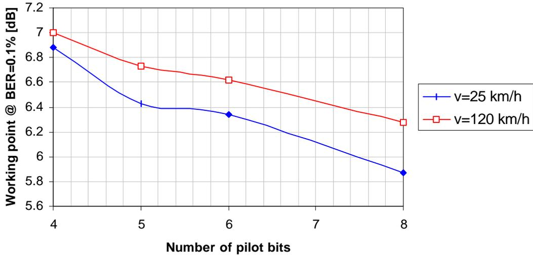
Fig. 1 System working point as a function of the number of pilot bits (uplink, Vehicular channel A)
