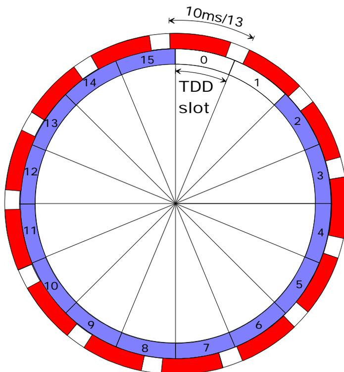
**figure 2 Example for a TDD to GSM alignment where only 2 idle TDD slots for monitoring (slot 0 and 1) are not sufficient to detect a complete FCCH burst (dark periods on the outer circle)**
