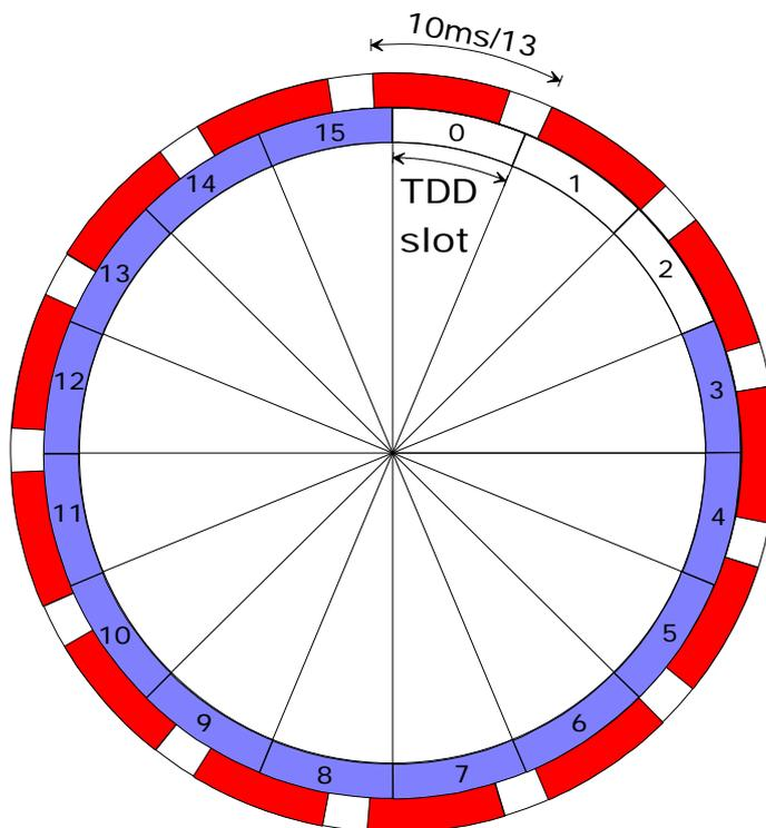
**figure 3 Example for a TDDtoGSM alignment with 3 idle TDD timeslots (slot 0, 1, 2) which can be used for monitoring GSM**
