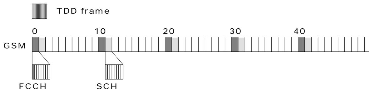
**figure 1 TDD frame and GSM multiframe structure**
