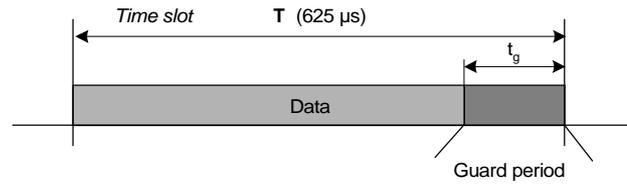
It is obvious that the tolerance of synchronisation also has an influence to the guard period  $t_g$ . Following inequality must be fulfilled, to avoid interference :
