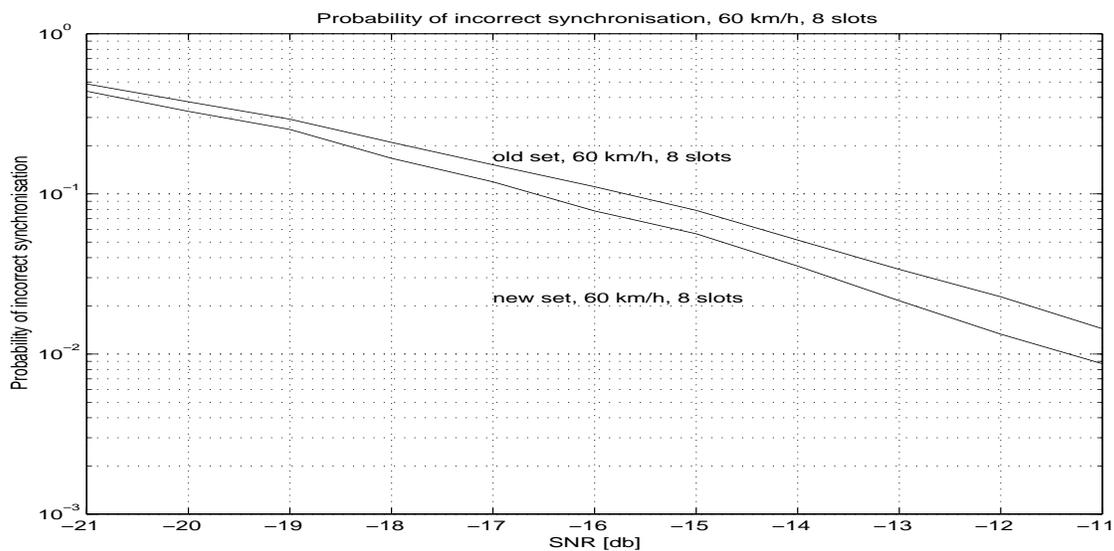
**Figure 11: Probability of incorrect code group/slot location synchronization in one ray Rayleigh fading vs. SNR, 8 slots integration, 60 km/h**
