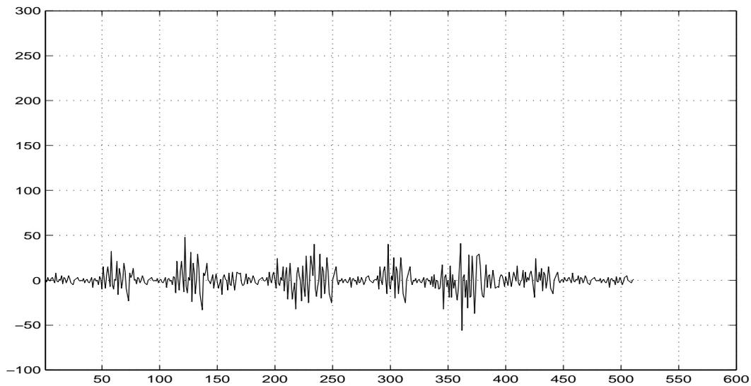
**Figure 7: Aperiodic cross-correlation of the Primary code with the cyclic hierarchical sequence (code group 2, slot 3)**
