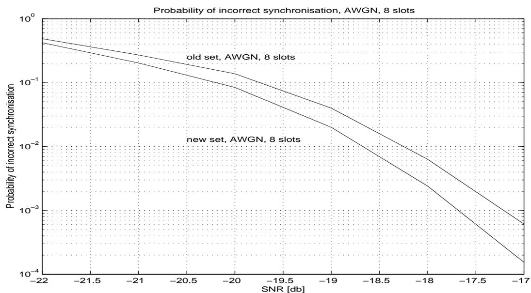
**Figure 10: Probability of incorrect code group/slot location synchronization in AWGN vs. SNR, 8 slots integration**
