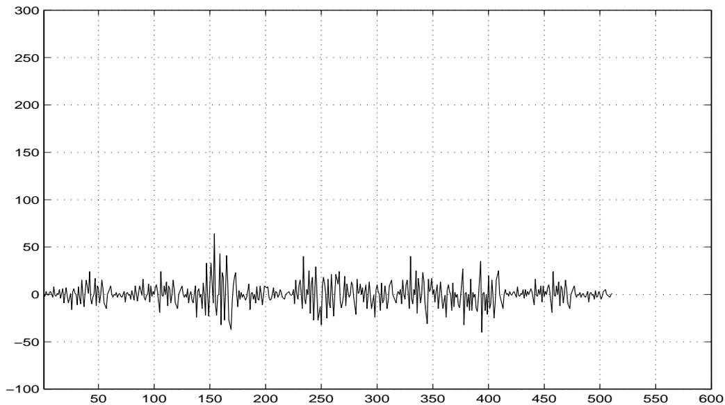
**Figure 6: Aperiodic cross-correlation of the Primary code with the cyclic hierarchical sequence (code group 2, slot 1= no cyclic shift)**
