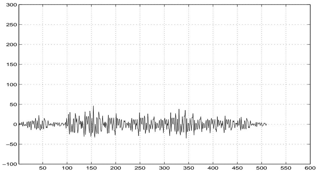
**Figure 8: Aperiodic cross-correlation of the Primary code with the cyclic hierarchical sequence (code group 22, slot 1= no cyclic shift)**
