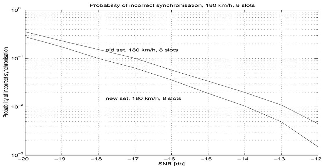
**Figure 12: Probability of incorrect code group/slot location synchronization in one ray Rayleigh fading vs. SNR, 8 slots integration, 180 km/h**
