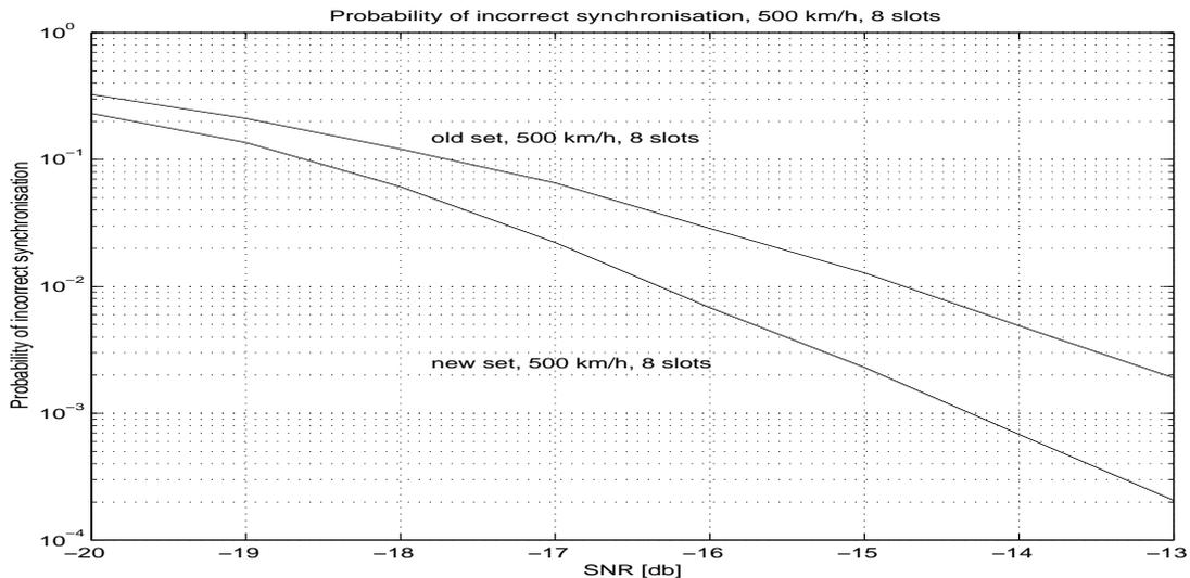
**Figure 13: Probability of incorrect code group/slot location synchronization in one ray Rayleigh fading vs. SNR, 8 slots integration, 500 km/h**
