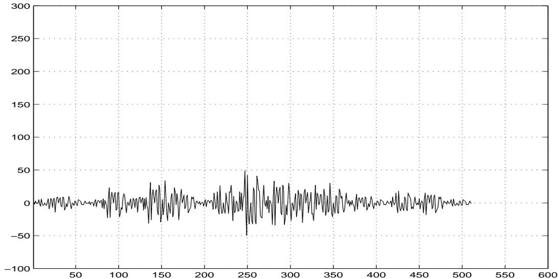
**Figure 9: Aperiodic cross-correlation of the Primary code with the cyclic hierarchical sequence (code group 22, slot 8)**
