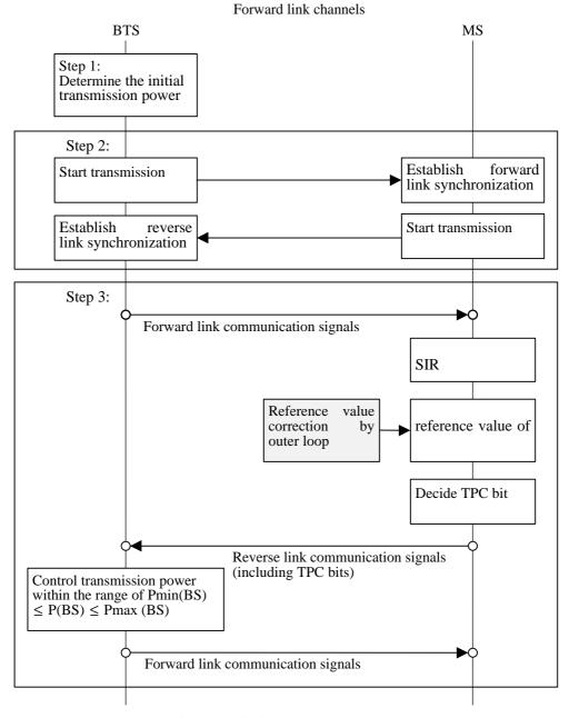
P(BS): Forward link transmission power Pmax(BS): Forward link maximum transmission power Pmin(BS): Forward link minimum transmission power
