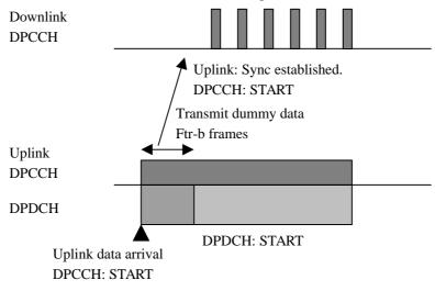
Figure 7: Transmission resumption of downlink DPDCH
