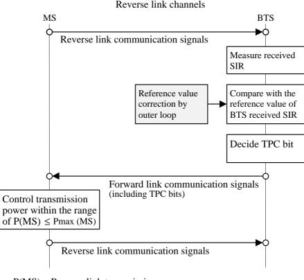
P(MS): Reverse link transmission power Pmax(MS): Reverse link maximum transmission power
