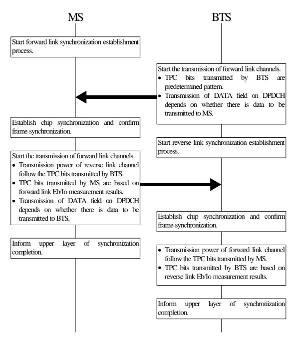
Fig.3.2.6-1 Synchronization Establishment Flow of Dedicated Channels
