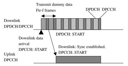
Figure 6: Transmission resumption of downlink DPDCH
