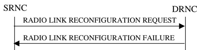
**Figure 15: Unsynchronised Radio Link Reconfiguration procedure, Unsuccessful Operation**
