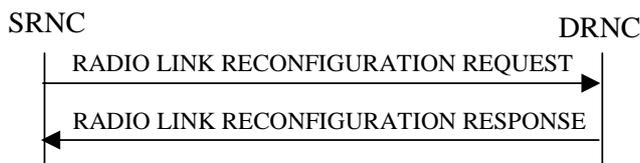
**Figure 14: Unsynchronised Radio Link Reconfiguration procedure, Successful Operation**
