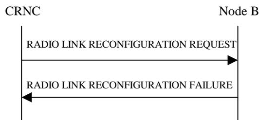
**Figure 35: Unsynchronised Radio Link Reconfiguration procedure, Unsuccessful Operation**
