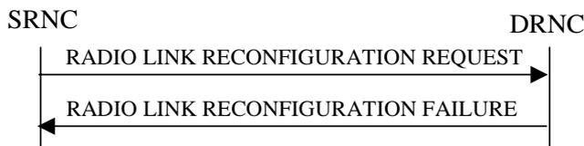
**Figure 15: Unsynchronised Radio Link Reconfiguration procedure, Unsuccessful Operation**
