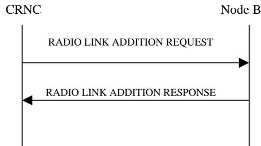
**Figure: 28 Radio Link Addition procedure, Successful Operation**
