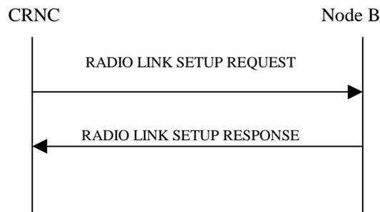
**Figure 24: Radio Link Setup procedure, Successful Operation**
