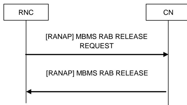
**Figure 8.2.yy: MBMS RAB Release Request procedure.**
