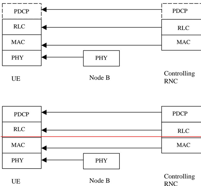
**Figure 5.3.1: Protocol Stack for MTCH**
