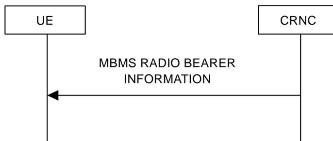
Figure 8.3.3: MBMS radio bearer information signalling flow
