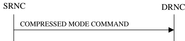
Figure 26: Compressed Mode Command procedure, Successful Operation
