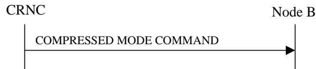
Figure 47: Compressed Mode Command procedure, Successful Operation
