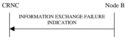
Figure 27P: Information Exchange Failure procedure, Successful Operation
