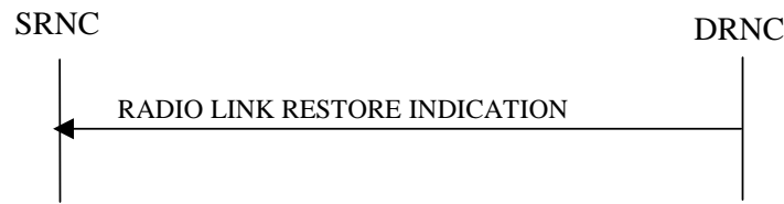
Figure 19: Radio Link Restoration procedure, Successful Operation
