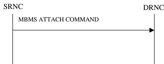
Figure x1: MBMS Attach procedure, Successful Operation
