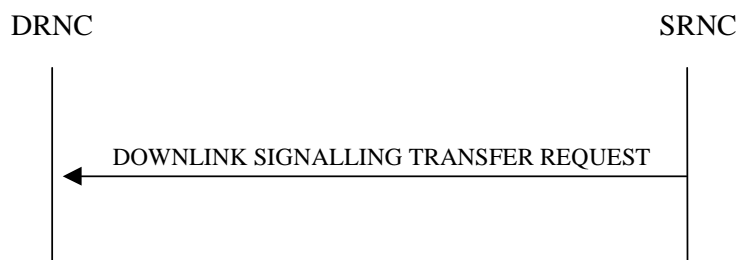
Figure 2: Downlink Signalling Transfer procedure, Successful Operation
