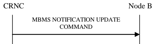
Figure x1: MBMS Notification Update procedure, Successful Operation
