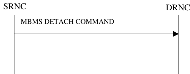
Figure x2: MBMS Detach procedure, Successful Operation
