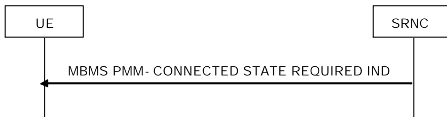
Figure 2727-25: MBMS PMM-CONNECTED state required indication signalling flow
