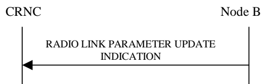
Figure 48: Radio Link Parameter Update Indication, Successful Operation
