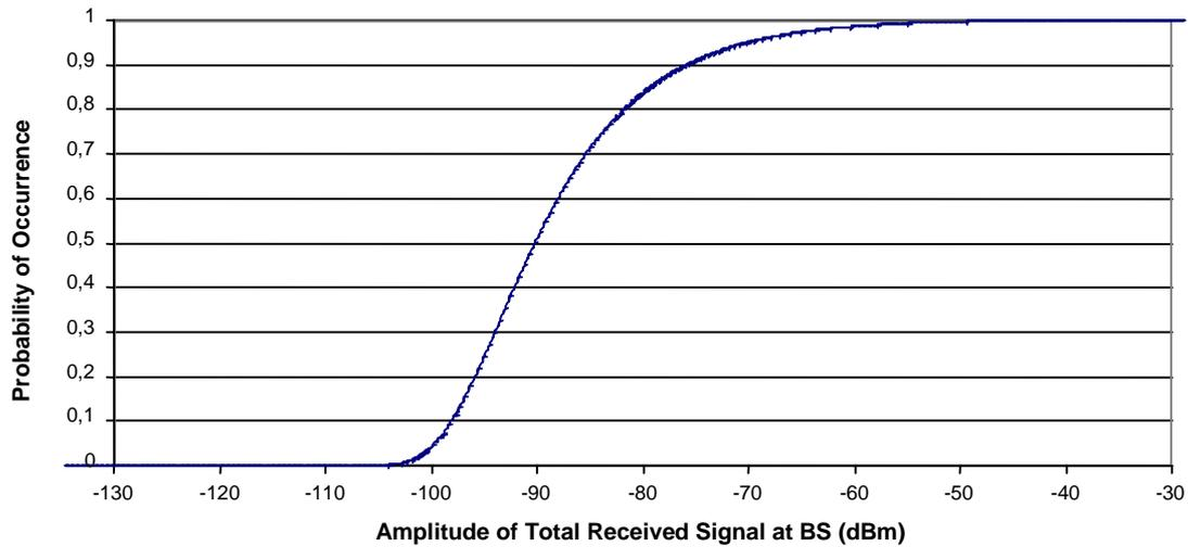
**Figure 26: CDF of Total Signal for Mixed Speech and Data System with 5 km Cells and Worst Case Geographic Offset**
