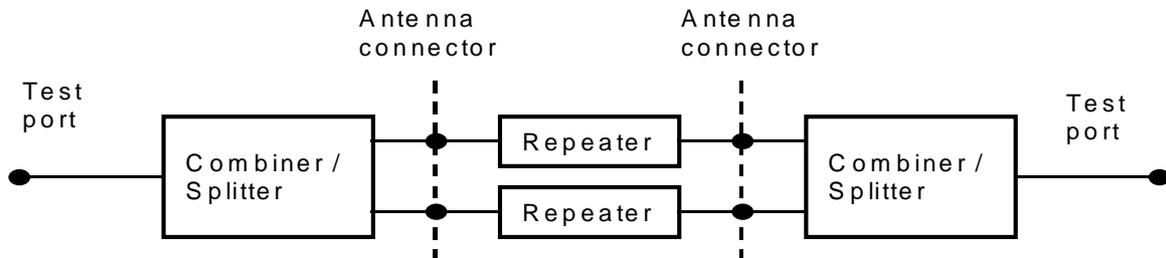
**Figure 5.6: Example of repeater configuration**
