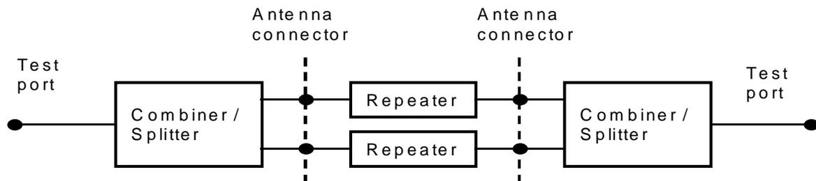
**Figure 5.6: Example of repeater configuration**
