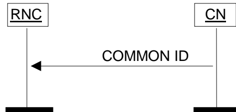
Figure 17: Common ID procedure. Successful operation.
