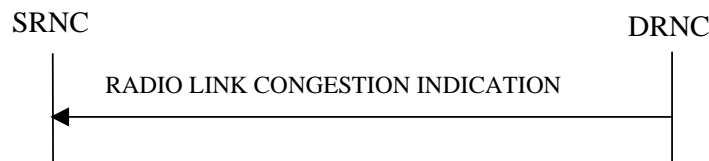
Figure 26C: Radio Link Congestion procedure, Successful Operation
