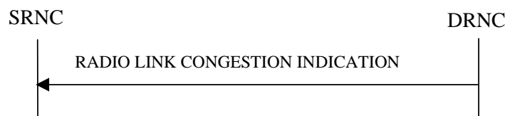
Figure 26C: Radio Link Congestion procedure, Successful Operation
