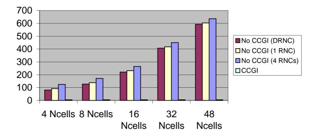
Fig.3: Accessed FDD cell with only FDD N-Cells: Number of bytes transferred of cell and neighbouring cell information on Iur vs. number of neighbouring cells with and without the CCGI mechanism.
