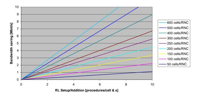
Fig.7: Bandwidth saving on Iur using the CCGI mechanism.
