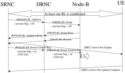
Figure 2: Use of separate TX activation
