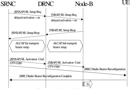
Figure 7: Use of delayed radio link activation
