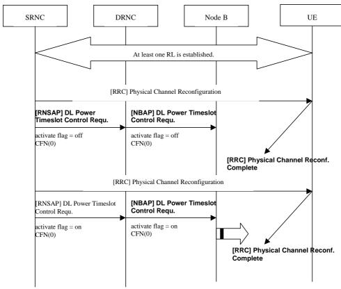
Figure 6: One-shot DL transmit power de-activation/activation(TDD)
