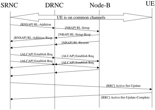
Figure 4: Signalling for RL-Setup (CCH to DCH switching)
