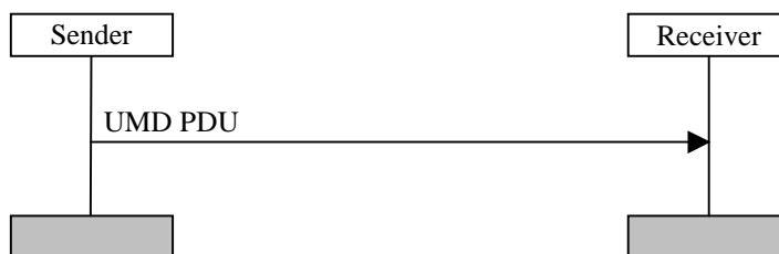
Figure 11.2: Unacknowledged mode data transfer procedure
